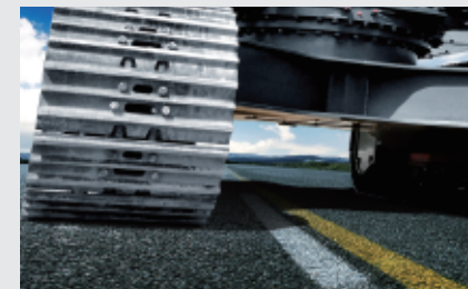
●加强的箱式结构车架全部由低应力，高强度钢板焊接而成 Strengthened chamber frame is totally welded by low stress and high strength steel plate ●标配全护板 Standard guard board
