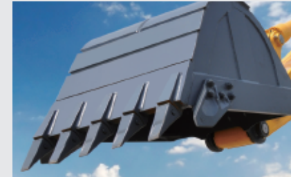
●铲斗使用加厚钢板，铲齿有效部分厚度和长度均得到有效加强，提高了铲齿的耐磨寿命。 Steel plate of bucket is thickened. The teeth have more wearing resistance due to their valid parts are thickened and lengthened. ●连接销应用烧结衬套，提高了耐磨性。 Connecting pin applies sintered sleeves and adds its resistance.
